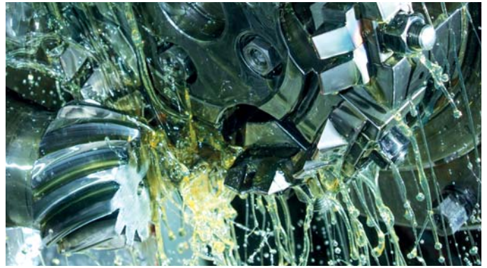
CNC Klingelberg C100U cutting machine for spiral gears
